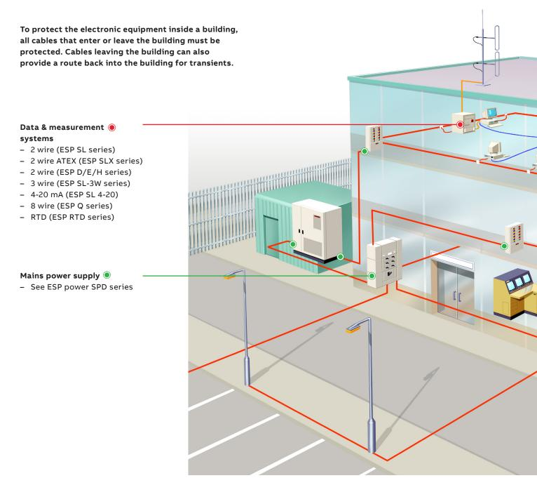
The comprehensive range includes protection for twisted pair data lines (including hazardous environments), computer networks, telecom systems including PBX and ISDN, CCTV, TV and RF systems.
