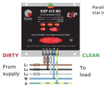
Parallel connection to three phase star (4 wire and earth) supplies
