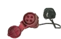
3 Phase adaptors Available in 16 & 32 Amp and 4 or 5 pin Configuration. Allows earth continuity and insulation resistance measurements to be made on 3 phase equipment using PAT testers with a standard UK 240V test socket. 16A 4 Pin Part No: 209A910 16A 5 Pin Part No: 209A911 32A 4 Pin Part No: 209A912 32A 5 Pin Part No: 209A913
