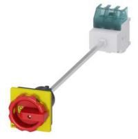
SENTRON, Switch disconnector 3LD, emergency switching-off switch, 3- pole, lu: 32 A, operating power / at AC-23 A 400 V: 11.5 kW, floor mounting with door coupling, rotary operating mechanism, Red / yellow, 4-hole mounting of the handle
