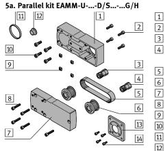
1 Lower part (1x)2 Screw (4x)3 Axis spring pin<sup>1)</sup> (1x)Motor clamping (1x)sleeve Toothed belt (1x)Toothed belt pulley (2x)Upper part (1x) (5x) Screw 9 (4x)Square nut Screw (4x)11 Centring ring<sup>2)</sup> (1x)
