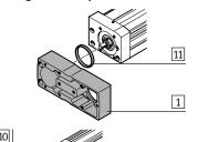
• Press the centring ring [11]2) into the drill hole in the lower part 1.
