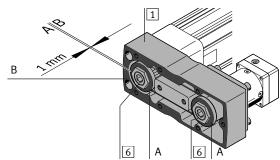
• Position surfaces (A) approx. 1 mm above the reference surface (B). Background: The tooth belt pulley 6 moves inwards when tightening.
