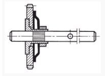
This device is situated inside the gearbox and is particularly recommended when gearbox protection is required in the event of accidental overloading.
