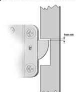
In the LOCKED position the distance between the RotoBolt bolt and the boltwork part that is moving the lock bolt should be approximately 1 mm.
