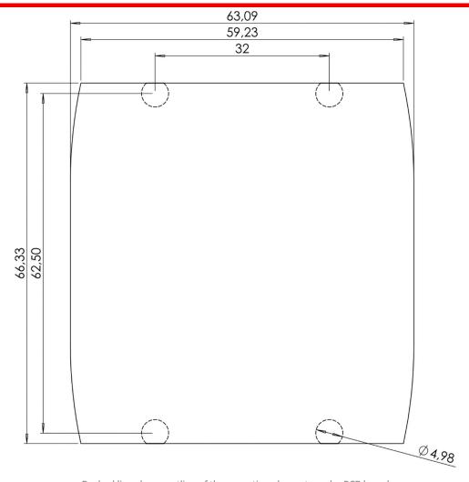
Dashed line shows outline of the mounting elements under PCB board Recommended mounting holes  $\varnothing 2,7$  All dimensions are given within +/-0,25mm tolerance
