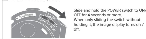
Slide and hold the POWER switch to ON/OFF for 4 seconds or more. When only sliding the switch without holding it, the image display turns on/off.
