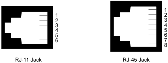
Figure 1: RJ-11 and RJ-45 Modular Pin Assignments
