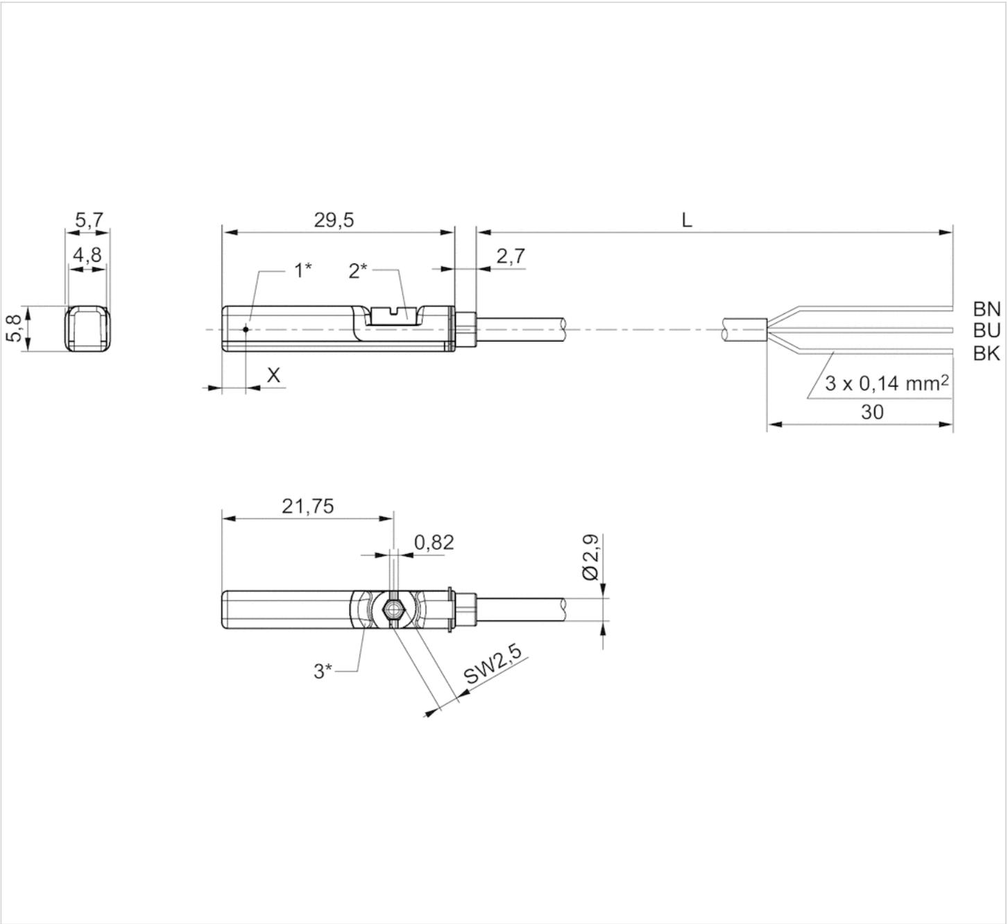
1\* = switching point 2\* = locking screw 3\* = LED window, transparent
