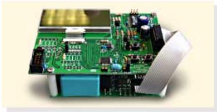
Metering reference design
