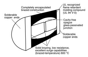
Fig. 1 - SUPERECTIFIER Construction
