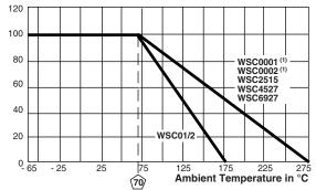
Note (1) As of 1/1/2010, WSC0001 and WSC0002 will be molded with thermoplastic and have the higher 275 °C temperature derating.
