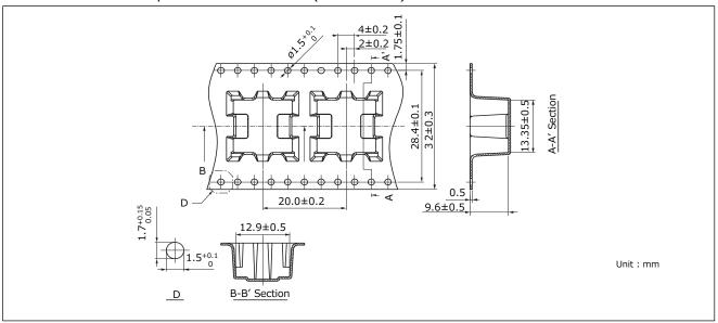
• Taping reel dimensions in mm (not to scale)
