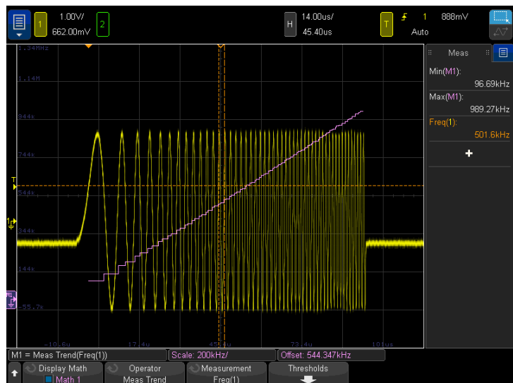
Figure 12. Measurement trend math function used to plot frequency versus time of a FM burst.
