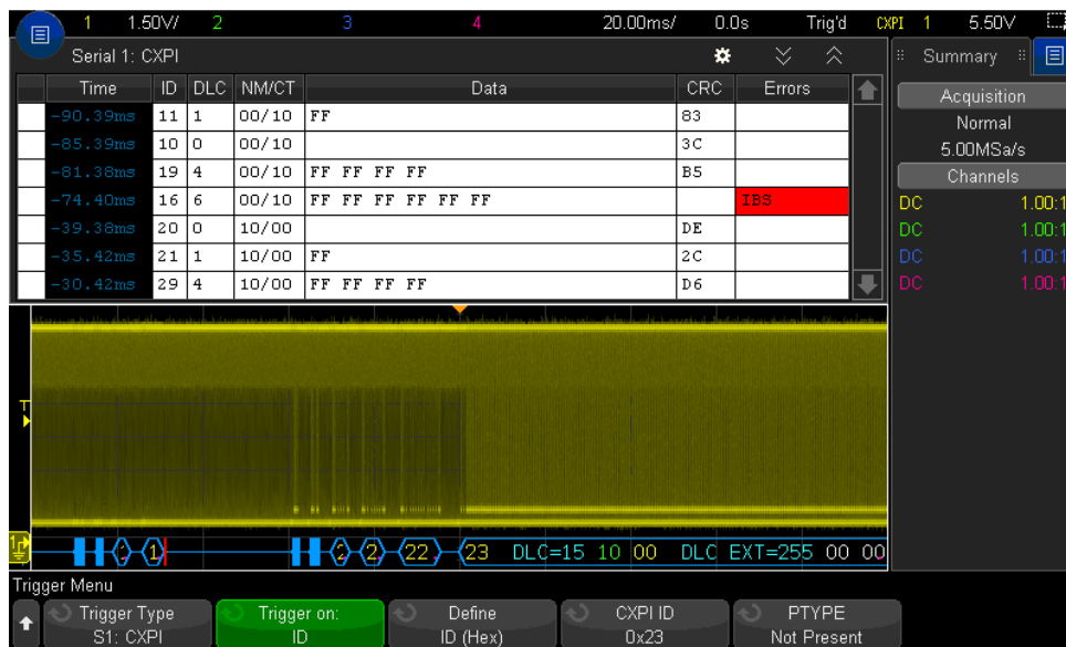
Figure 9. CXPI decode on an InfiniiVision X-Series oscilloscope.
