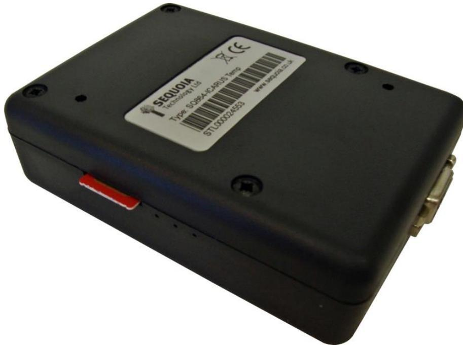
**Figure 4: Incorrectly inserted SIM**
