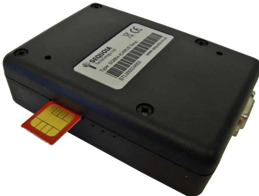
**Figure 2: Inserting the SIM**
