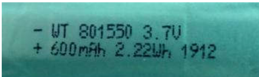
电池组铭牌 View of the battery nameplate
