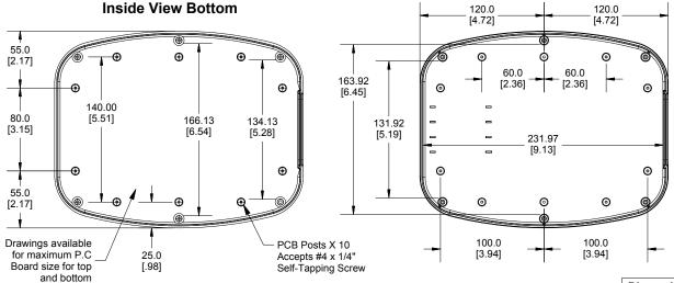
Purchased assembly includes top and bottom cover, 1 removable panel and 6 cover screws (M3-0.5 x 18mm), M3 Brass inserts are installed for cover screws, Enclosure molded from FR ABS (UL94-V0) plastic.
