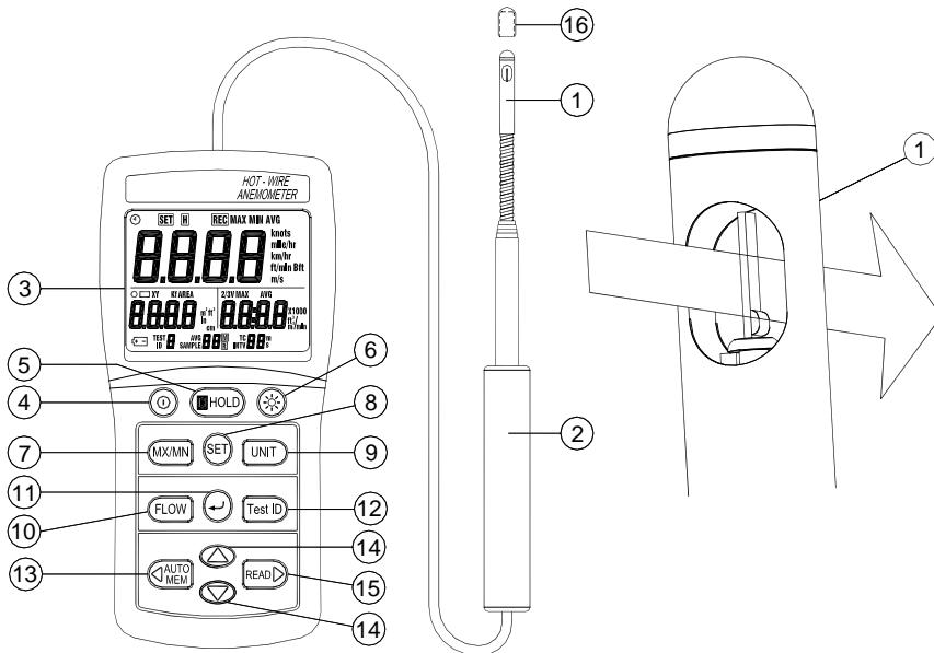
1. Air velocity sensor. (Measurement direction)
