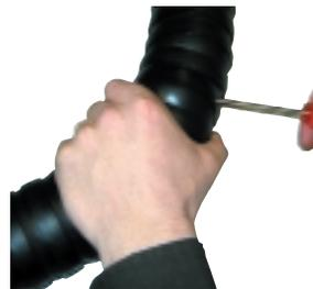
3. Push screwdriver through perforated window, moving chain links to the maximum bending position on the opposite side
