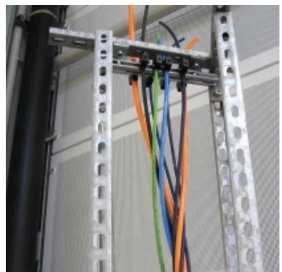
Test 2: CF Robot; more than 2,454,600 movements tested okay in long term test.
