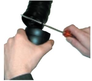
4. Remove socket from ball using the screwdriver as a lever.
