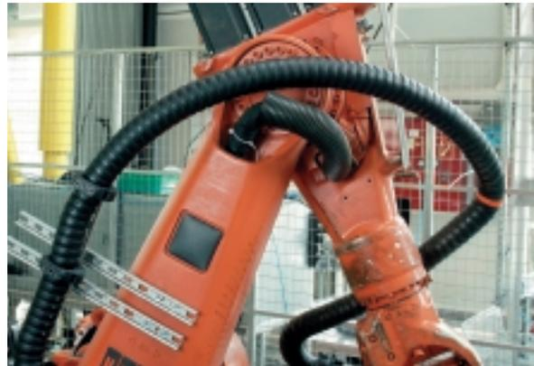
Application with premounted fiber rod element TRC-F-1800-1-0 from the red line with Triflex® R TRC-70-110-0 (without fiber rod).
