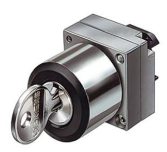
22MM ROUND METAL ACTUATOR: RONIS LOCK WITH 2 KEYS MAINTAINED CONTACT 2 SWITCH POSITIONS O-I LOCK NUMBER 421, REMOVE O+I WITH HOLDER POSSIBLE SPECIAL LOCKS FOR RONIS KEYSWITCHES: SB31, 455, 421
