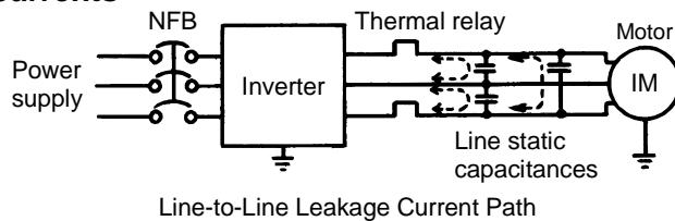
Line-to-Line Leakage Current Path
