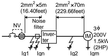
Example of leakage current per 1km in cable path during commercial power supply operation when the CV cable is routed in metal conduit (200V 60Hz)
