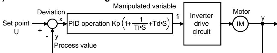
Kp: Proportional constant    Ti: Integral time    S: Operator    Td: Differential time
