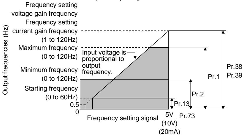
**Relationships between Frequency Setting Inputs and Output Frequencies**
