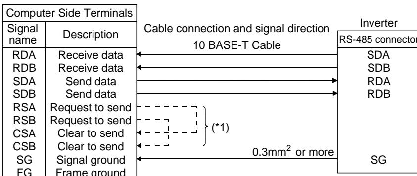
2) Wiring of one RS-485 computer and "n" inverters (several inverters)
