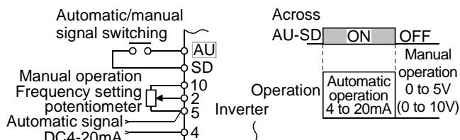
When the 4-20mA signal is used to perform operation, always short the AU signal.
