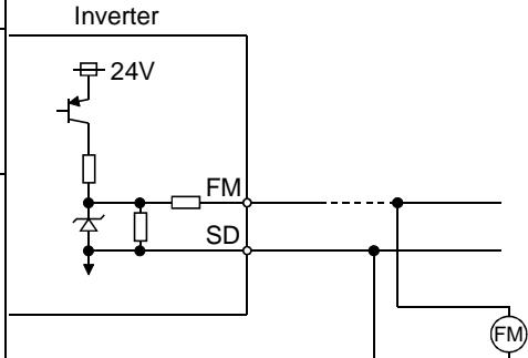
Example of Inverter and Frequency Meter
