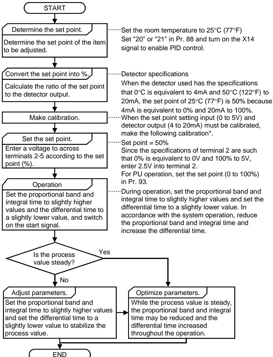
\*When calibration is required, use Pr. 38, Pr. 39 and calibration parameters C2 to C7 to calibrate the detector output and set point setting input in the PU mode during an inverter stop.
