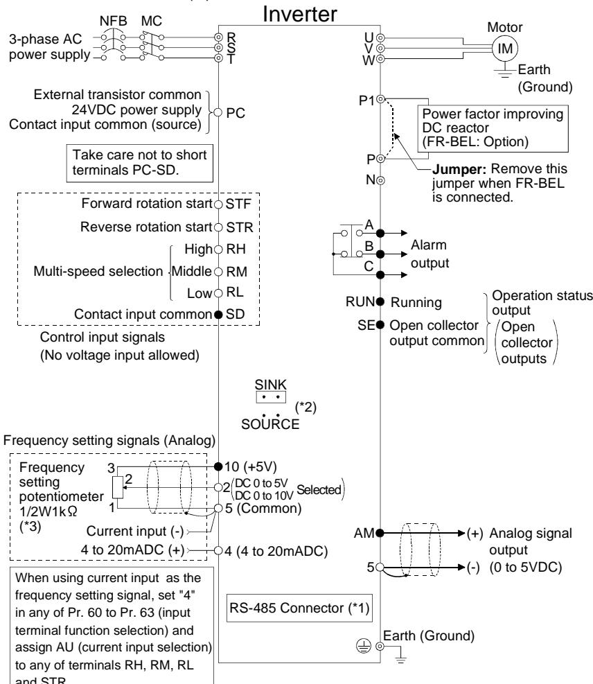
© Main circuit terminal ○ Control circuit input terminal ● Control circuit output terminal
