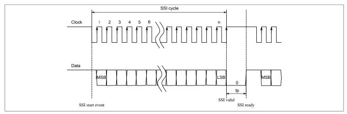
The SSI cycle is normally configured to network event 225 "AOSISOP". This ensures that the new encoder position is available for the next " $I/O \rightarrow Synchronous$  frame" transfer. It is important to note the SSI transfer time and the X2X cycle time since the SSI cycle must be completed within this time frame.
