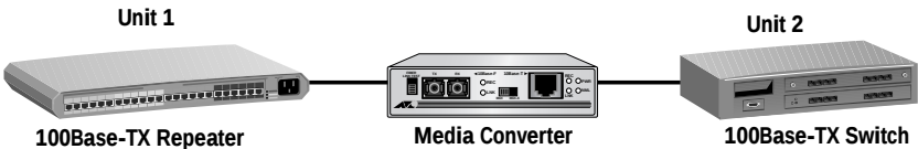
Figure 1 Example of a Duplex Mode Mismatch
