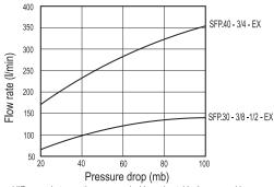
(difference between the pressure inside and outside the reservoir) SFP+F-EX
