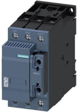
capacitor contactor, AC-6b 75 kVAr, / 400 V, 3-pole, 110 V AC, 50 Hz, auxiliary contacts: 1 NO + 1 NC, screw terminal, size: S2
