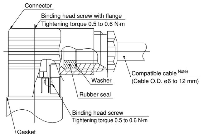
Note) For an outside cable diameter of  $\phi 9$  to 12 mm, remove the internal parts of the rubber seal before using.
