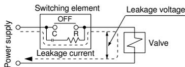
DC coil: 2% or less of rated voltage
