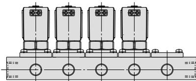
Enter the product's part number in order, counting the 1st station from the left in the manifold arrangement, when viewing the individual port in front.
