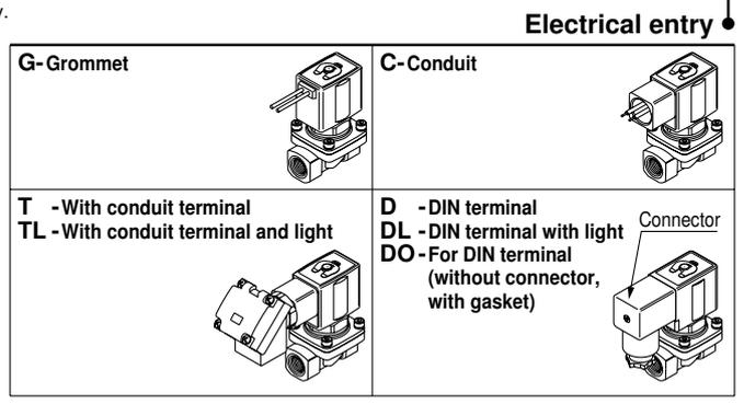
\* Refer to Table (3) for available combinations between electrical option (L) and rated voltage.
