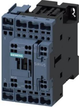
power contactor, AC-3, 25 A, 11 kW / 400 V, 4-pole, 48 V DC, main contacts: 2 NO + 2 NC, auxiliary contacts: 1 NO + 1 NC, spring-loaded terminal, size: S0
