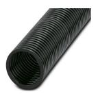
Protective hose, material: PA 6, UV-resistant: yes, flexible, degree of protection: IP68, color: black, flammability rating in acc. with UL 94: HB, inside diameter: 36 mm, Total length: 25 m
