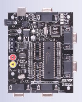
Both analogue and digital data is gathered through Ghost ICT and displayed on the Flowcode Softscope. For communications busses, decoding overlays for UART, SPI and I2C are available. Ghost data can also be passed to simulations/SCADA components in Flowcode to provide Human Machine Interface style debug features.
