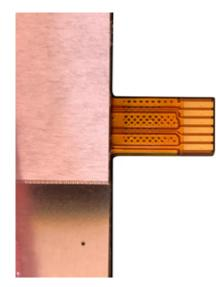
Remove any packing foam and tape to release the Touch control board from the back of the display. Place the display face up and line up the small USB connector PCB.
