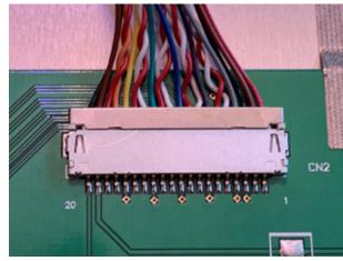
The connection should look like this when the connector is connected correctly.
