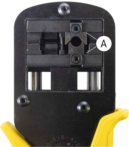
Fig. 15: Change of shielding crimping sets
