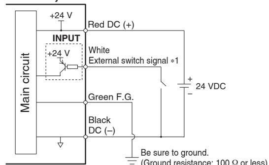
\*1 The external switch signal is used in an OR configuration with the trigger input. When the external switch signal is not used, cut back the semi-strip wire to prevent any contact with the conductor.
