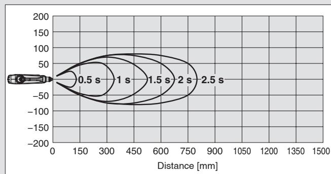
2) Supply pressure: 0.1 MPa Flow rate consumption: 119 l/min (ANR)
