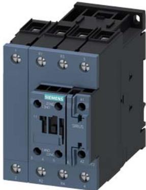
power contactor, AC-3, 35 A, 18.5 kW / 400 V, 4-pole, 42 V AC, 50 Hz, main contacts: 2 NO + 2 NC, auxiliary contacts: 1 NO + 1 NC, screw terminal, size: S2
