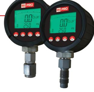
Optional Minimess® Male or Female adaptor to allow for easy hand tight connection / disconnection to Minimess® test points or hoses (max working pressure 630 bar).
