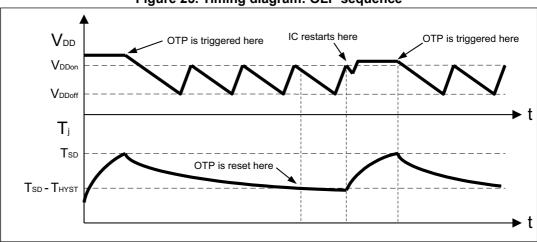
Figure 25. Timing diagram: OLP sequence
