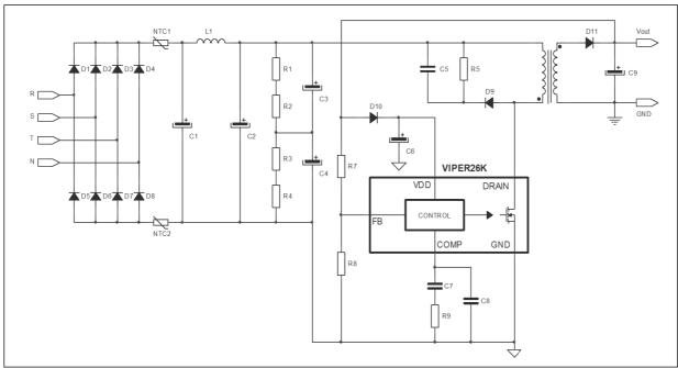
Figure 28. Typical non isolated flyback configuration
