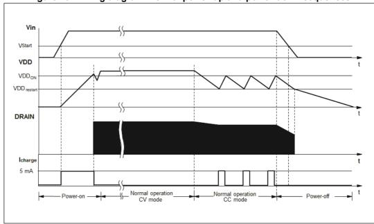
Figure 20. Timing diagram: normal power-up and power-down sequences
