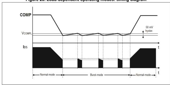
Figure 23. Load-dependent operating modes: timing diagram
