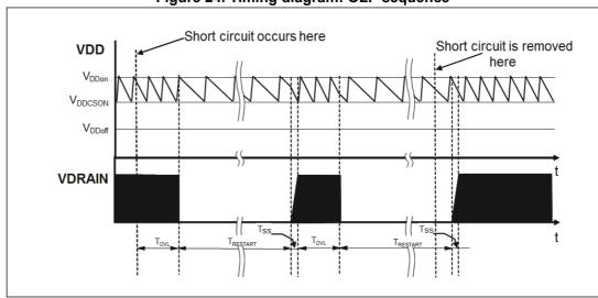
Figure 24. Timing diagram: OLP sequence
