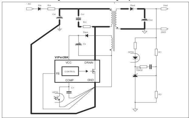
Figure 30. Recommended routing for flyback converter
