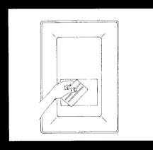
Excess liquid should then be squeegeed from the middle out with the PA1 applicator covered with a HB104 Applicator pad.
