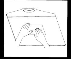
Lay the material with the glossy side up (the side exposed to the UV) onto the Peeling Board. Remember which was the corner between the two masked edges. Smooth out the film onto the adhesive covered Peeling Board.
