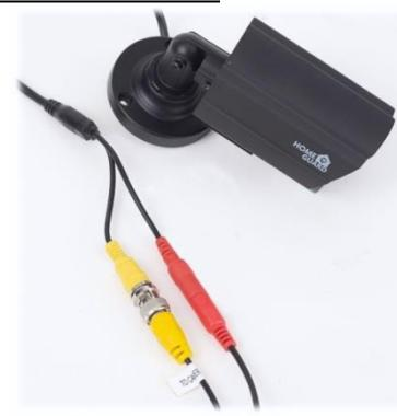
Connect the CCTV cable(s) video lead to the DVR in each Video Input port as required. Ensure you use the connector marked "For DVR side only"
