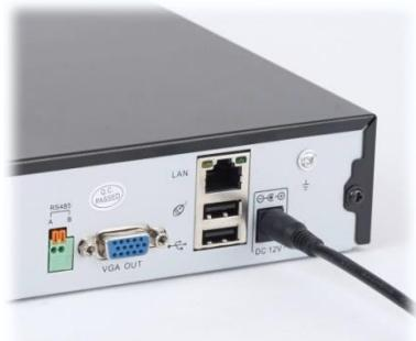
Connect the DVR power supply (marked “**For DVR use only**”). Do not connect it to mains power at this stage.
