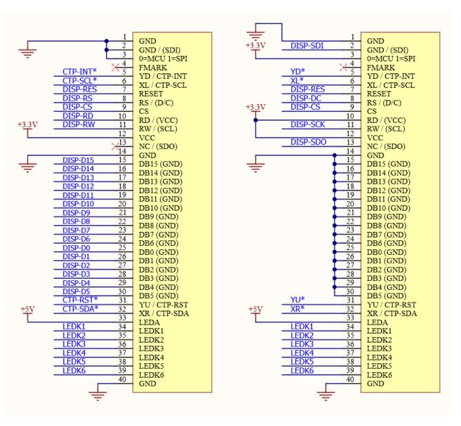
Note the pinout of this 3.5" display differs from the pinout on 2.4", 2.8" and 3.2" displays, for just the SPI Mode (Pin8 and Pin11), so if working with 2.4", 2.8" and 3.2" displays in the 4DLCD family, take note that the MCU mode pinout is the same and backwards compatible, but SPI pinout is not identical.
