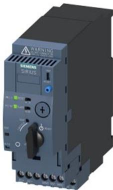
SIRIUS Compact load feeder DOL starter 690 V 110...240 V AC/DC 50...60 Hz 8...32 A IP20 Connection main circuit: plug-in, without terminals Connection auxiliary circuit: screw terminal
