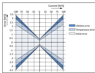
Figure 3 Distribution of max. total error in S1 range
