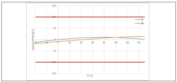
Figure 9 Typical offset drift over temperature
