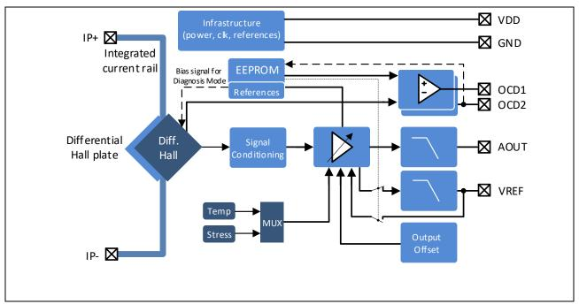
Figure 2 Block Diagram
