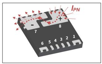
Figure 1 Pin layout PG-TISON-8-5 The current  $I_{PN}$  is measured as a positive value when it flows from pin 8 (+) to pin 7 (-) through the integrated current rail.
