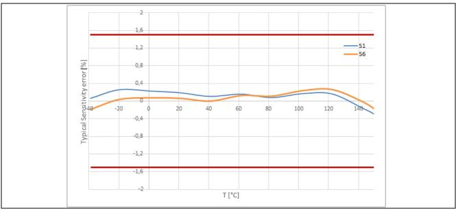
Figure 8 Typical error in sensitivity over temperature
