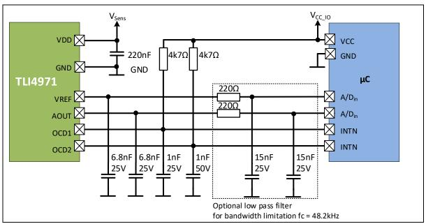
Figure 7 Application circuit with external components
