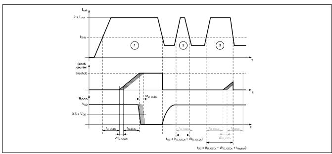
Figure 4 Fast over-current detection output timing
