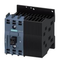
Solid-state contactor 3-phase 3RF3 AC 53 / 9.2 A / 40  $^{\circ}\text{C}$  48-480 V / 24 V DC 2-phase controlled Instantaneous switching Spring-type terminal
