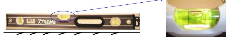
**Step 3.**Spin the Level 180 Degrees on the Same Leveling Surface
