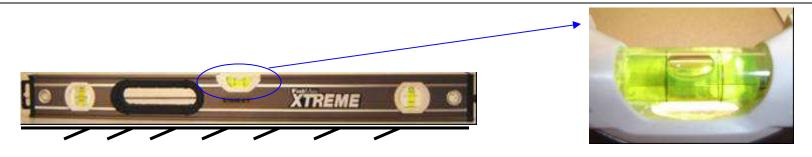
**Step 1.**Put the level on any flat surface. It's not necessary that the surface be level.
