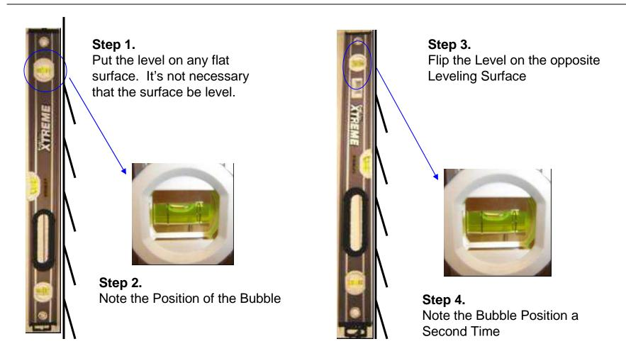
**Result**: As long as the bubble is in the same position for both level orientations, then the level is accurate.
