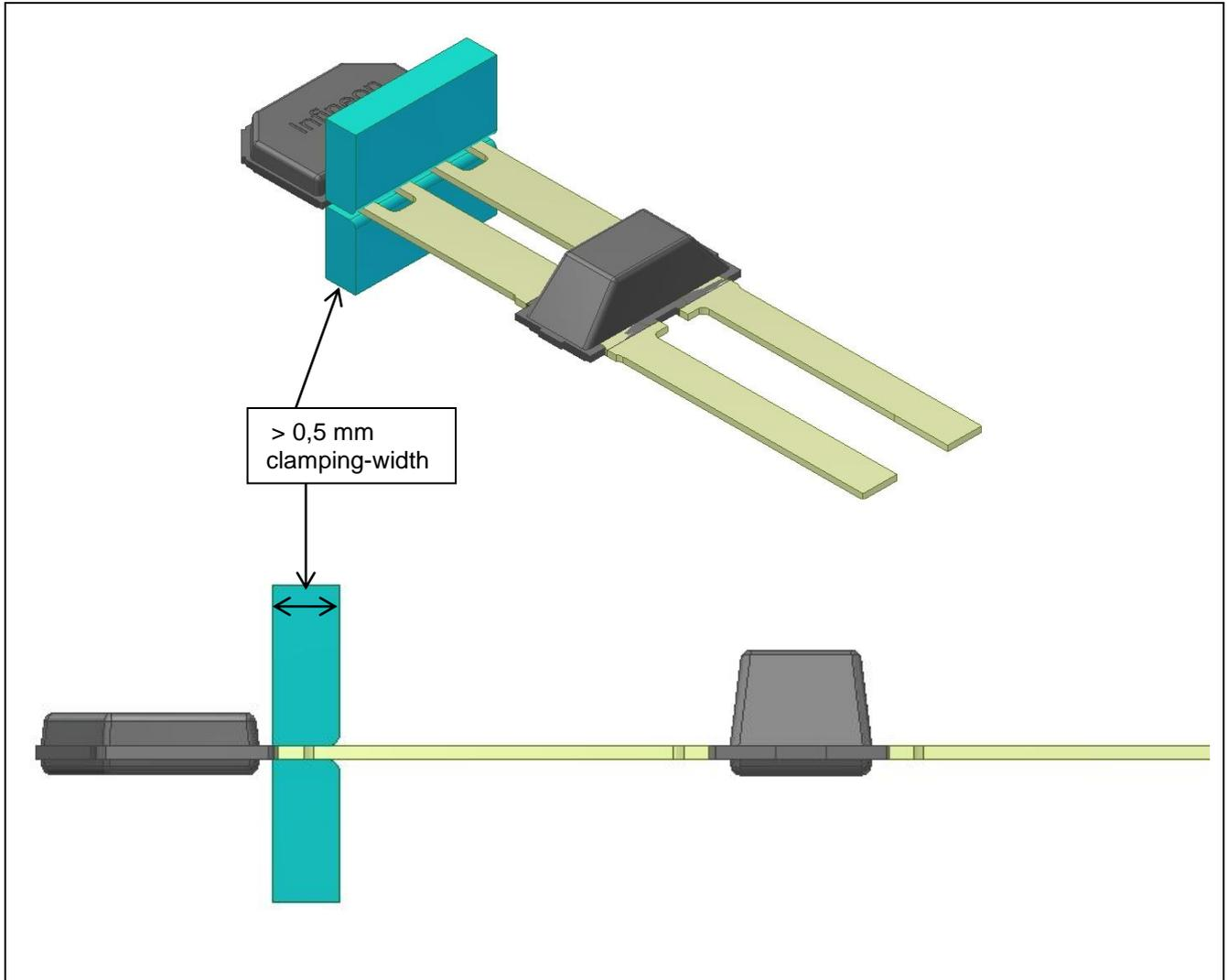
**Figure 4 Explanation of Clamping Procedure**
