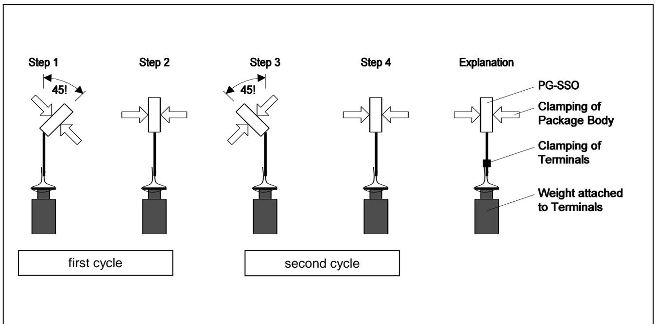
Figure 6 describes the international standard IEC 68-2-21 bending procedure.
