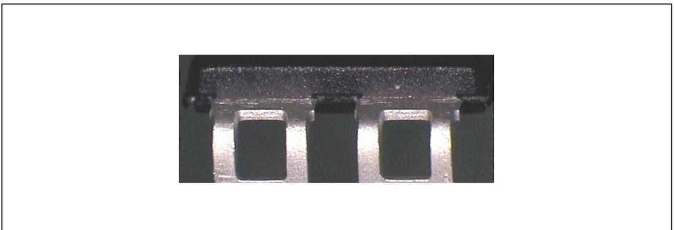
**Figure 5 Figure show a good 90 degree bent device..**
