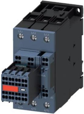
power contactor, AC-3e/AC-3, 51 A, 22 kW / 400 V, 3-pole, 24 V DC, 0.8-1.2\* Uc, with integrated varistor, auxiliary contacts: 2 NO + 2 NC, main circuit: screw terminal, control and auxiliary circuit: spring-loaded terminal, frame size: S2, suitable for PLC outputs, captive auxiliary switch
