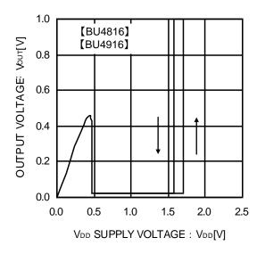
Fig.7 Operating Limit Voltage
