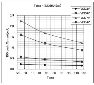
Fig.19 Current Consumption vs. Power Supply Voltage
