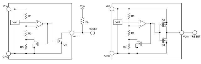
Fig.12 (BU48xx type internal block diagram)
