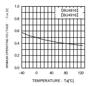
Fig.11 Operating Limit Voltage
