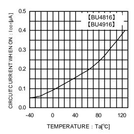
Fig.9 Circuit Current when ON
