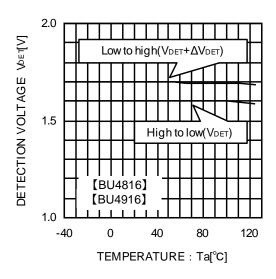
Fig.8 Detecting Voltage Release Voltage
