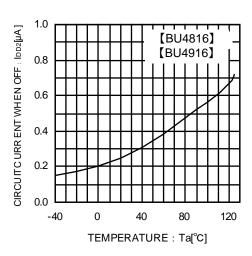
Fig.10 Circuit Current when OFF
