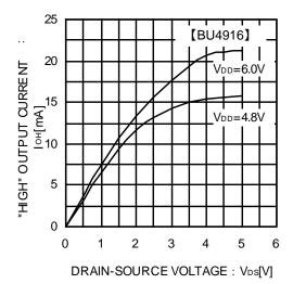
Fig.5 "High" Output Current
