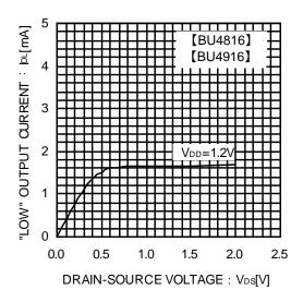
Fig.4 "LOW" Output Current
