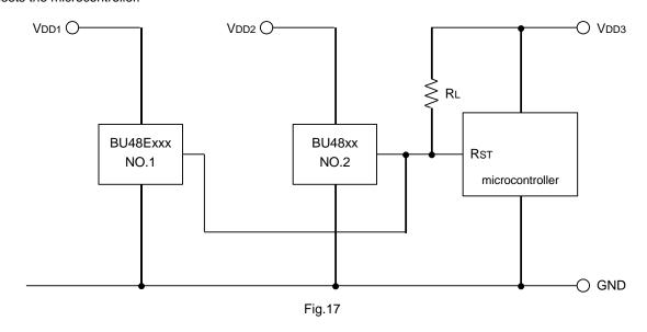
To reset the microcontroller when many independent power supplies are used in the system, OR connect an open drain output type (BU48xx series) to the microcontroller's input with pull-up resistor to the supply voltage of the microcontroller ( $V_{DD3}$ ) as shown in Fig. 20. By pulling-up to  $V_{DD3}$ , output "High" voltage of micro-controller power supply is possible.
