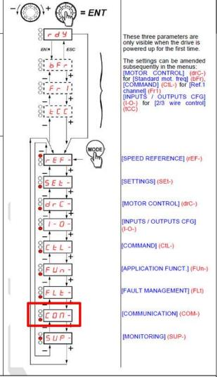
For the drive to operate with the new parameters, a power cycle (on, off, on) is required.
