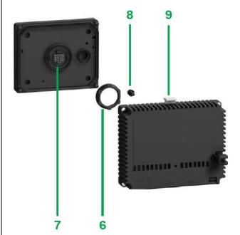
A Magelis STU Small Panel is made up of a front module (comprising the screen) and a rear module (comprising the CPU plus terminals and connectors). The two modules are fixed together by means of a hole measuring 22 mm in diameter. The fixing system contains the following elements:
