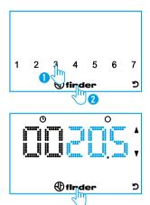
Repeatedly press the Finder button to step through and display the hours together with the appropriate set temperature.
