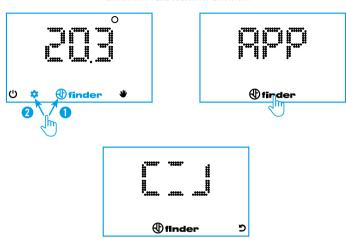
In the case where the APP credentials were not inserted by the expiry of the timeout, the Chronothermostat performs a RESET of the configuration and the internal Wi-Fi is turned off.
