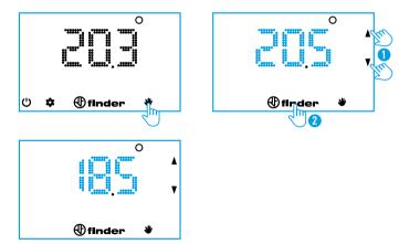
To exit the manual setting and return to the main screen, press the "hand" button.
