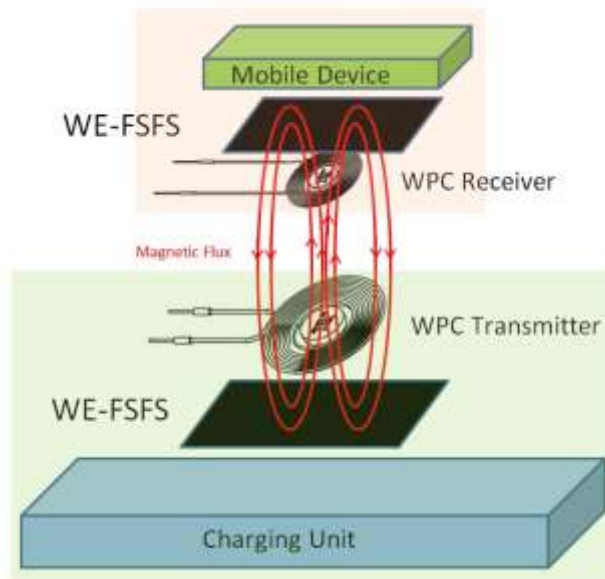
Figure 7 Wireless power with shielding
