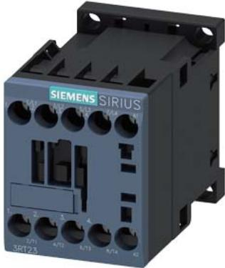
Schütz AC-1, 18 A, 400 V / 40 °C, 4-polig, AC 24 V, 50/60 Hz, Schraubanschluss,
